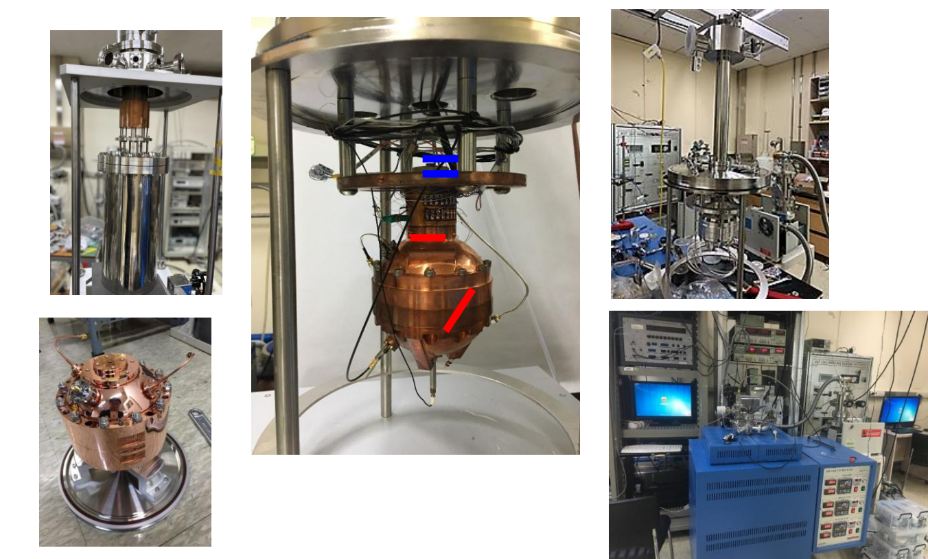
low temperature high temperature <Acoustic gas thermometry setup at KRISS>
