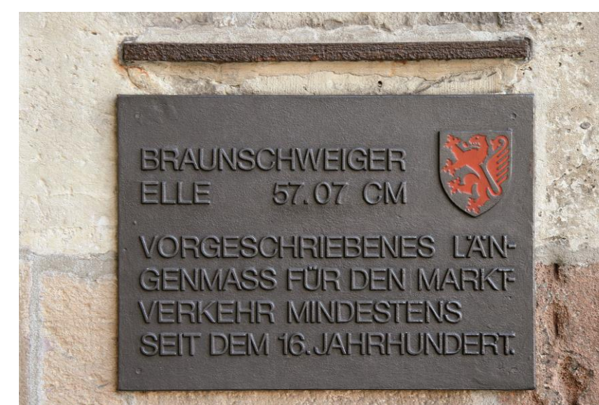
Fig. 4: Local length standard (Braunschweiger Elle) to be used on the market place close to the Old Town Hall in the city of Braunschweig in Germany.
