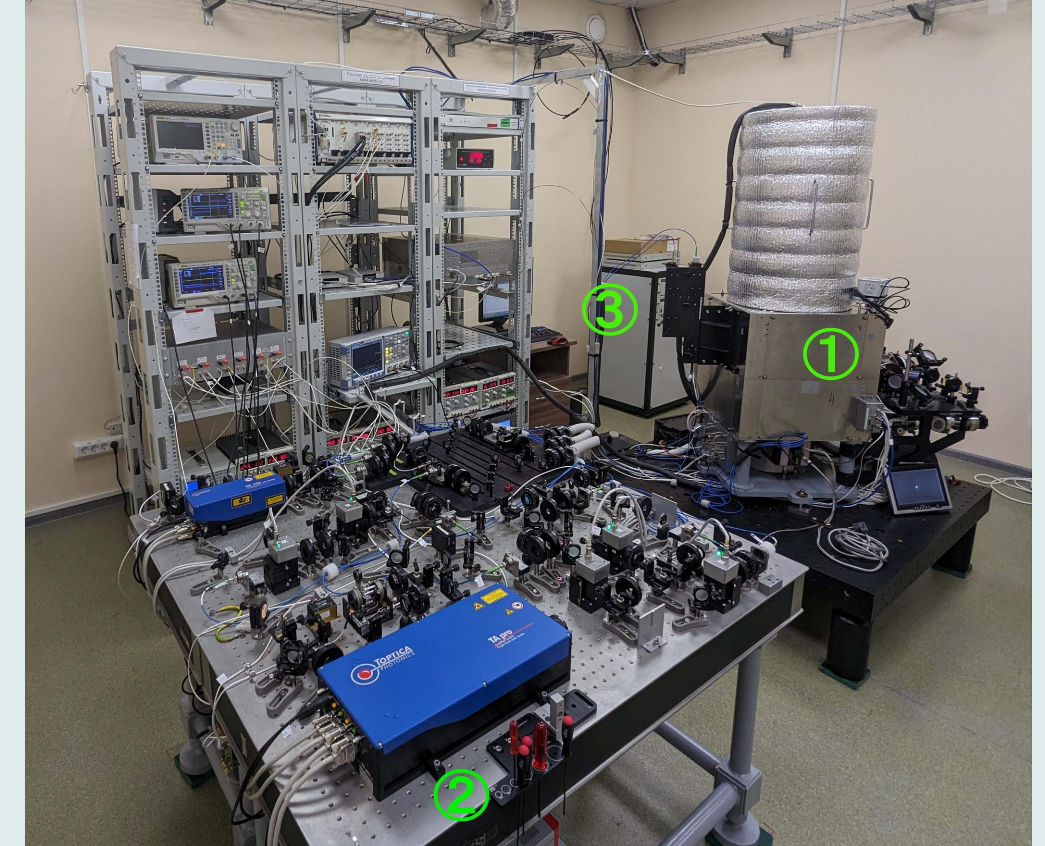
Fig. 6 Rubidium atomic fountain (Rb5): 1 – physical package, 2 – laser system, 3 – microwave source
