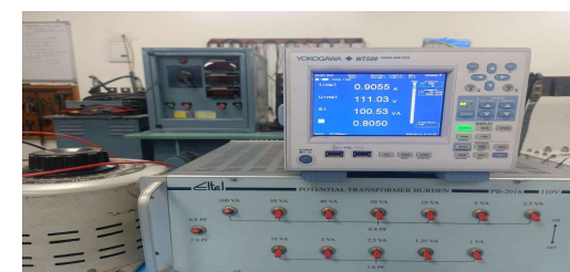
Experimental setup: PT burden calibration
