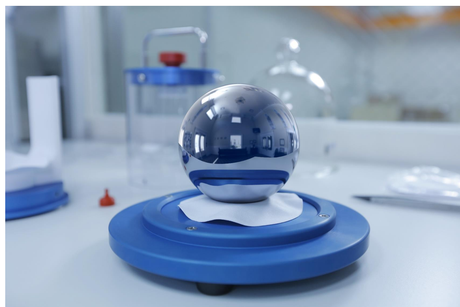
Fig.1 The ^{28}\text{Si} -enriched sphere "Sikg2803a" at CMS/ITRI
