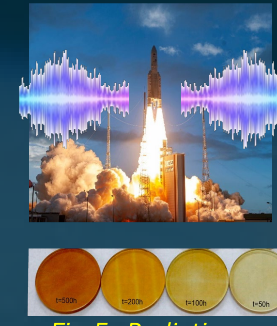
Fig 5: Radiation damage to glass
