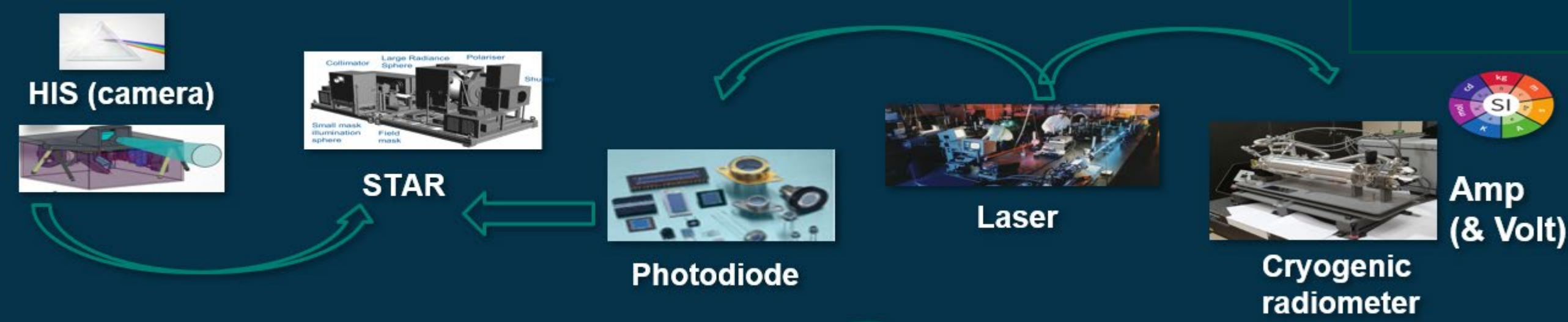
Fig 11a: Terrestrial pre-flight calibration traceability chain from cryogenic radiometer to instrument (HIS) using a tuneable laser. The STAR is an NPL facility incorporating a tuneable laser and integrating sphere for deployment in a clean room to calibrate sensors under vacuum.
