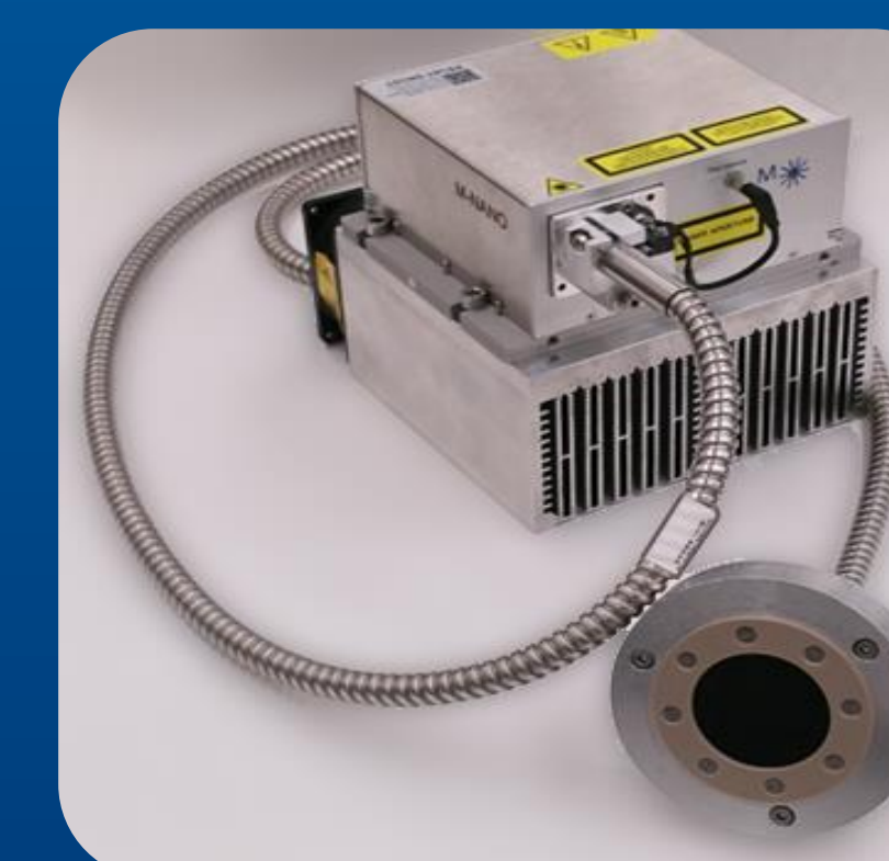
Figure 4: NPL's Photoacoustic Source, a laser-generated ultrasound emitter that is capable of producing a broadband, continuous, frequency response up to 100 MHz. The device further works at close range, removing the need for time consuming alignment and minimising spatial averaging corrections.
