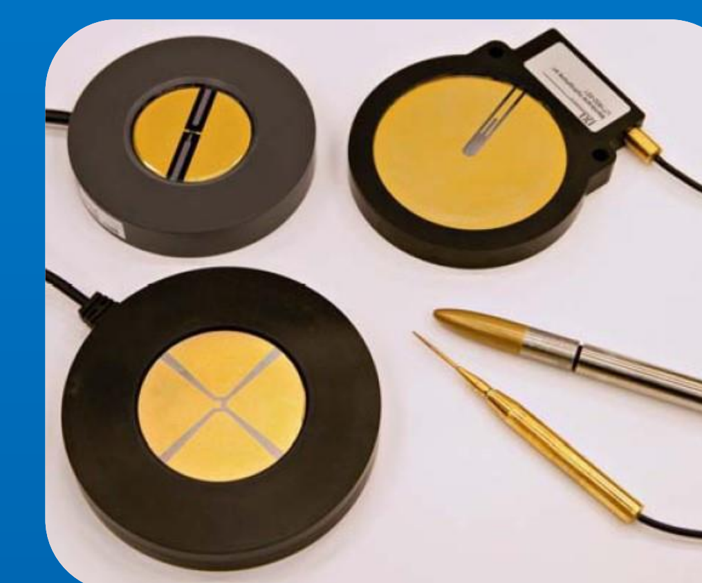
Figure 2: Example hydrophone devices from different manufacturers. Hydrophones can detect the real-time acoustic pressure fields generated by medical devices. The three large devices are of membrane type, the mainly-silver cylinder is a capsule or golden-lipstick type, and the gold cylinder is a needle type.
