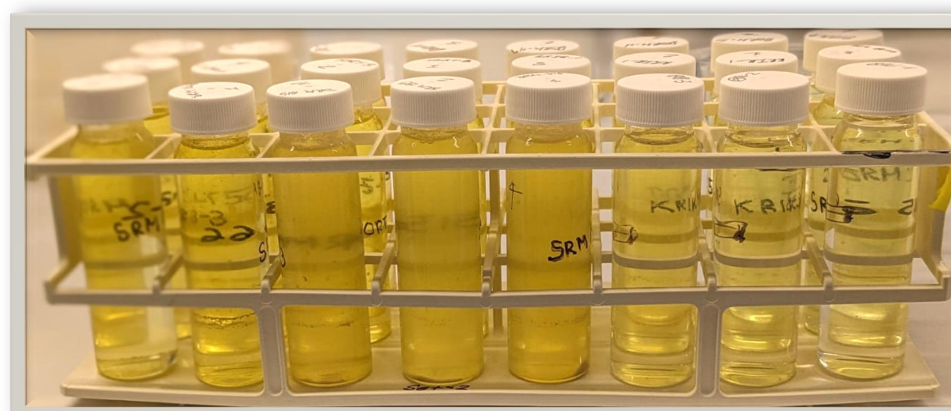
Tissue samples following the modified EPA Method 1631 digestion protocol and dilution with 0.5% BrCl
