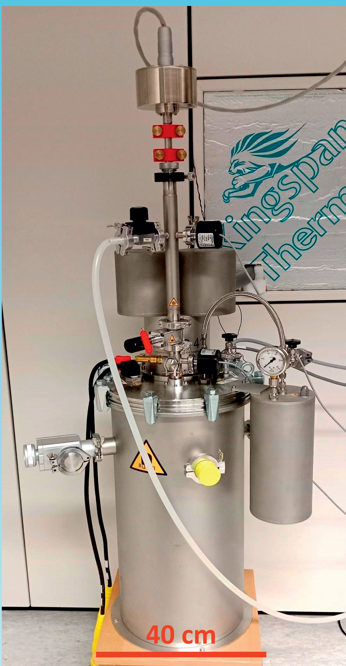
Image of a tabletop cryocooler system that is used for graphene-based quantum Hall resistance (QHR) measurements at PTB.
