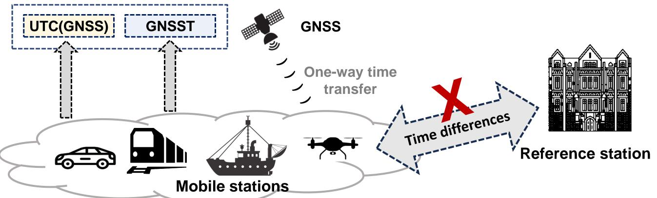
To ensure the metrological traceability of the time and frequency values obtained by the mobile stations, a study on time transfer in dynamic scenarios should be conducted.
