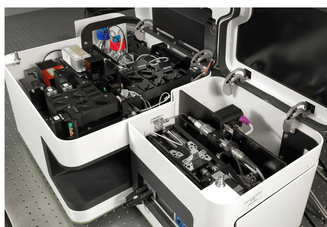
Gas buffered device. Despite use of pressure and temperature sensors the uncertainty for the volume is higher: typically u_{rv} = 0.25\%
