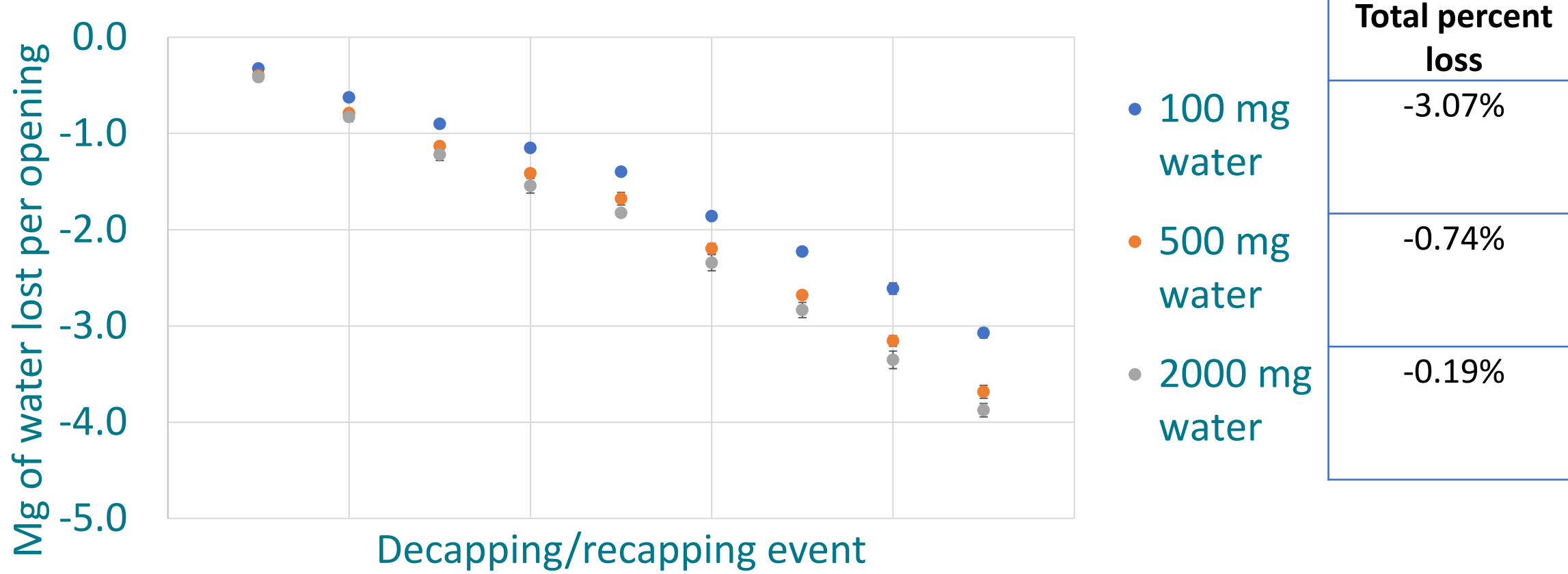
Evaporation of water from 10 mL vial after opening the lid, waiting 2 minutes and closing the lid
