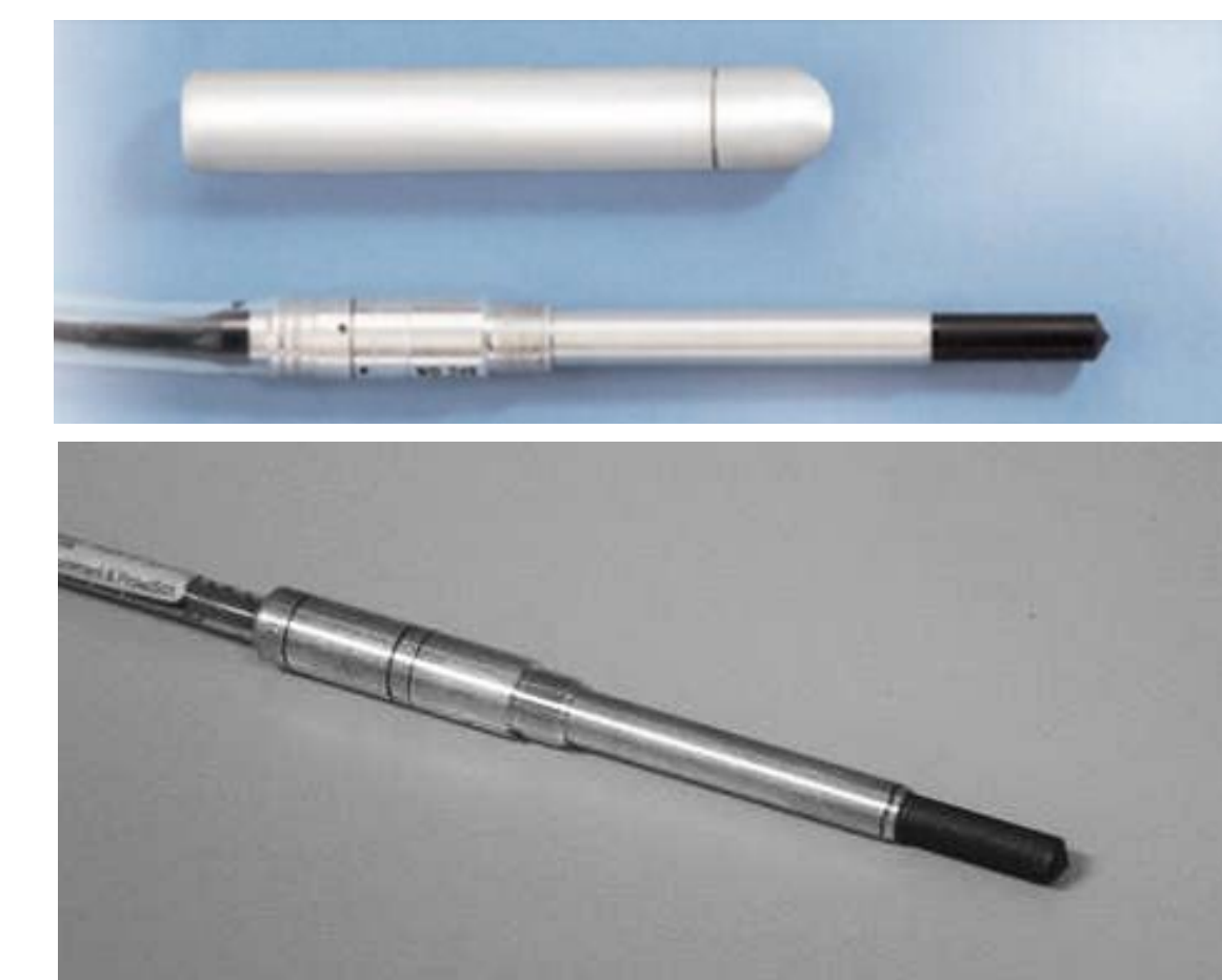
The Farmer chambers IBA FC65-G and NE2571 used for measurements in air and in water.
